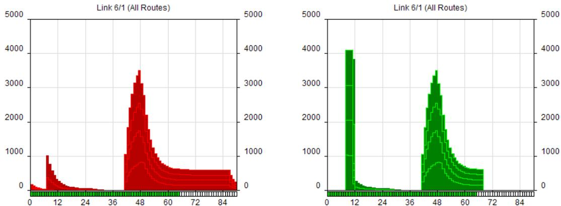
Each Route Flow Profile is shown as a separate 'layer' in the graph. The layered Route Flow Profiles cannot be shown on a combined inflow/outflow graph as the display becomes extremely complex and difficult to understand.
