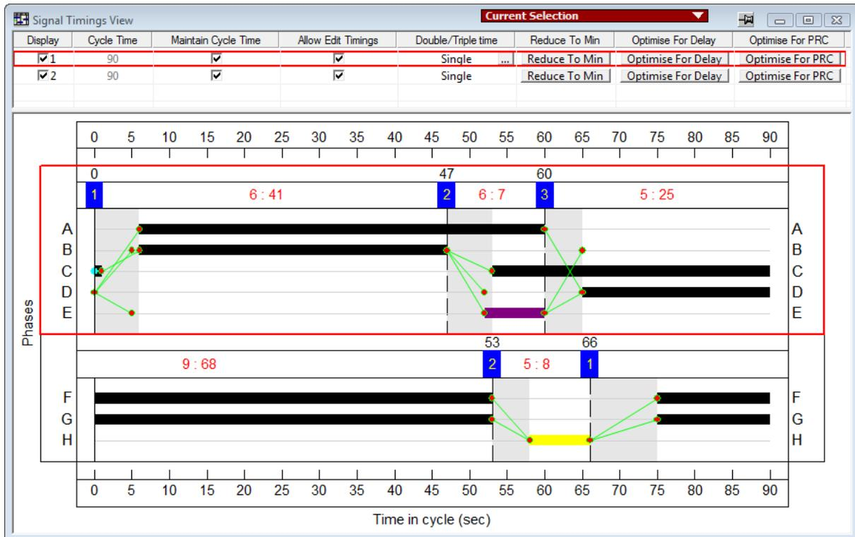
As well as viewing Stage and Phase timings, the Signal Timings View also shows detailed Interstage structure, Stage Minimums and allows signal timing optimisation of individual Controllers or Stage Streams to be carried out.
