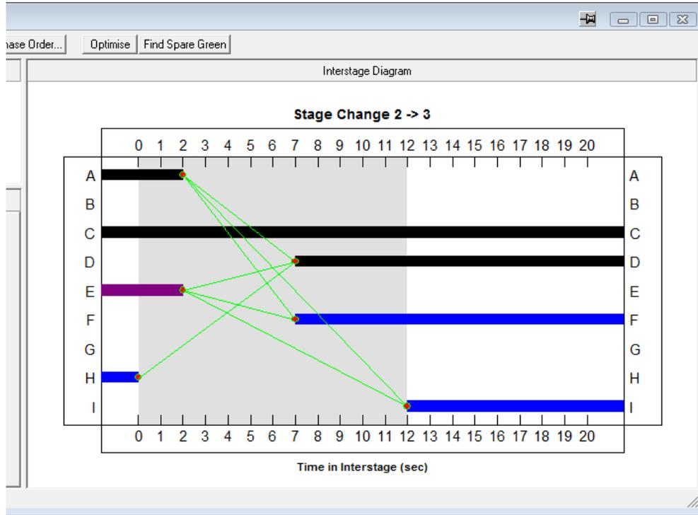
The Interstage Diagram initially accommodates Interstages up to 20 seconds and marks the time axis every two seconds. This can be changed if necessary by double clicking on the time axis and entering a new size and scale as appropriate. If necessary LinSig will adjust the time axis markings to avoid overlapping.
