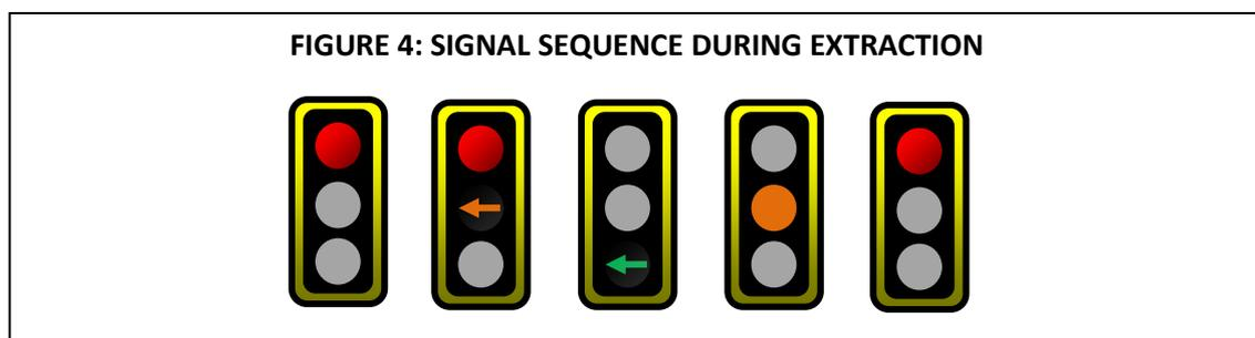
2.14. If the non compliant vehicle is in Lanes 1 or 2, which is normally the case, Lanes 3 and 4 can continue to operate but if the non compliant vehicle is in Lane 3 or 4 all traffic northbound traffic flow has to be stopped to extract the vehicle.
