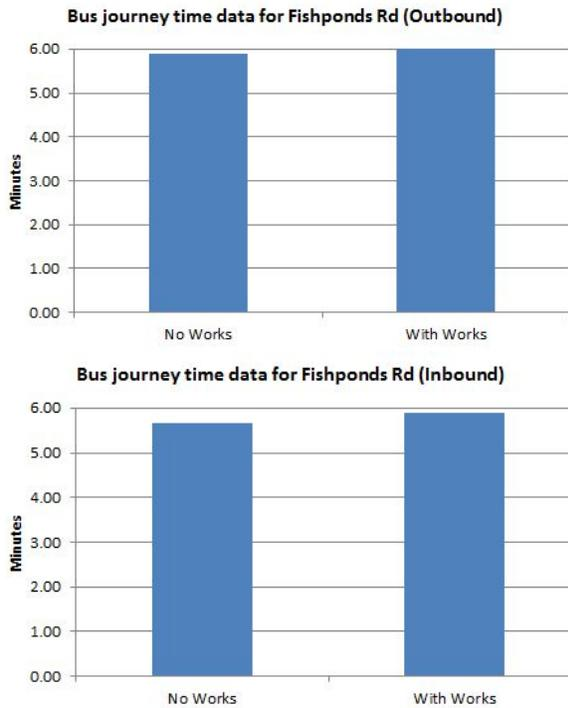
*This low impact was likely to be partly due to the reduced traffic flows at the start of the school holidays and partly due to the improved coordination between the sets of signals. Overall, on-site operatives and control room staff observed that the UTC temporary signals were noticeably more effective than the usual local control method and made the traffic flow more smoothly.*
