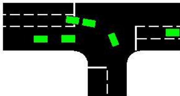
LinSig uses the give way model described above to model the capacity of the right turn during the period it is opposed by oncoming traffic. Common practice in the UK for many years has been to use Tanners formula to calculate the amount of traffic turning in gaps. This can be closely approximated in LinSig 3 by using 1440 for Intercept and 1.09 for slope in the give way model.
