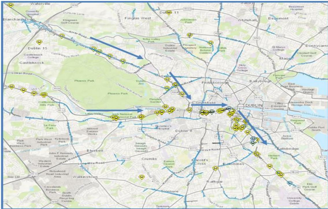
**Figure 12 Centralised Bus Priority System displaying in real-time, the location of all buses servicing one Stop, for a single point in time on the North Quays. (Each icon represents a bus location)**
