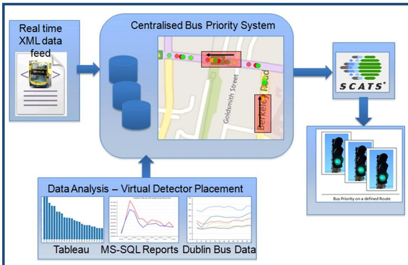
Figure 1 - Component Architecture of the Centralised Bus Priority System
