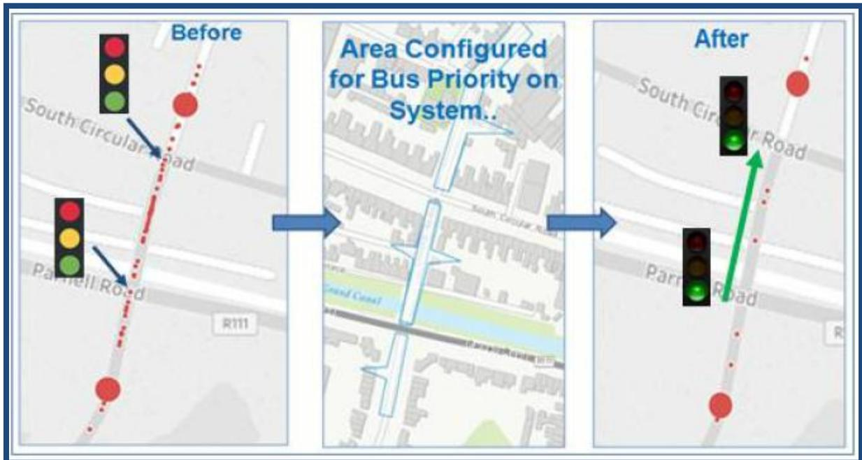
Figure 5 – Data driven placement of virtual detectors for bus priority.
