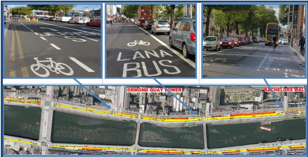
Figure 13 Bus Priority changes within the City Centre, traffic reduced to one lane.
