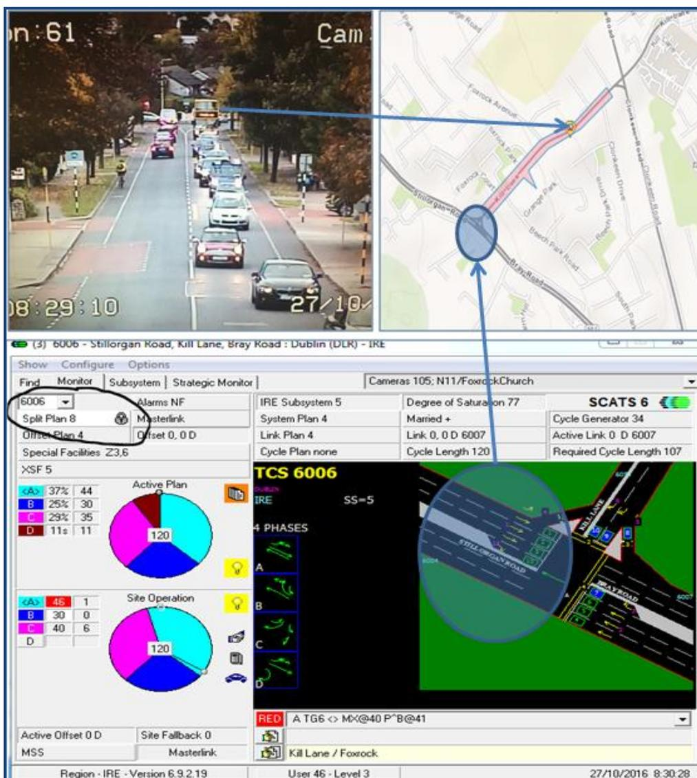
Figure 6 Example of Priority Call via virtual detector.
