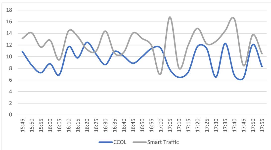
**Figure 4 – Average delay time for cyclists, in seconds**
