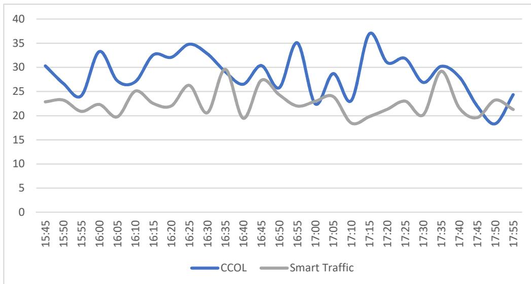
**Figure 3 – Average delay time for car traffic, in seconds**
