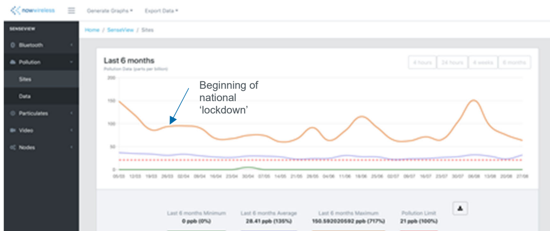
Figure 5: Report from Senseview displaying the data for all locations over the last six months, again a drop can be seen at the point of 'lockdown'
